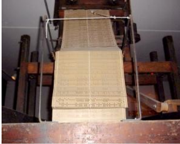
Jacquard loom with punch cards ca. 1840 from Smithsonian NMAH , photo by Steven E. Schoenherr
