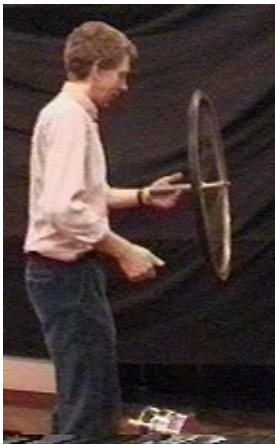
Figure 10: Do-it-yourself bicycle wheel gyroscope!
